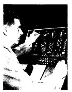
shorts, indicating which ones are bad and where. Operating principle of the tester is based on the fact that the main switch box is the heart of a plane's circuit.
