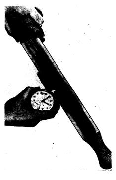
watches must be wound each day, it has a real practical advantage. The device is a strip of fabric-backed polyvinyl plastic on a paddle a foot long. Along this, the winding stem is drawn in one motion. Science News Letter, May 22, 1943
