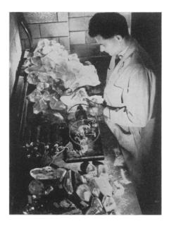
TESTING QUARTZ — This shipment of quartz crystals from Brazil is being inspected with the aid of an arc lamp in the Electronics Laboratory of General Electric. Thin slices of the quartz crystals will be used to keep radio stations on their assigned frequencies.
