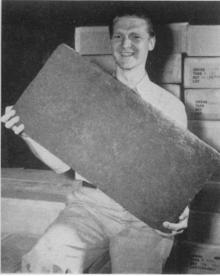
RUBBER—At a new buna S synthetic rubber plant in West Virginia, this rubber is being produced for use in tires and tank treads. When the Government-owned plant is in full production, enough rubber to make 63,000 tires will be produced daily. At the left is shown the rubber after removal of the electrical charges causes the particles to stick together. At the right rubber has been dried and pressed into loaves.
