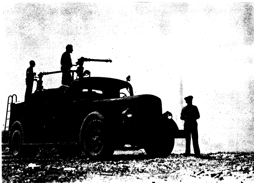
CRASH TRUCK —Built for Army Air Forces, this truck is ready to rush to the scene of a crash and shoot hundreds of gallons of water on a burning plane, blacking out the fire and rescuing pilot and crew. Engineers of Mack Trucks, Inc., worked with the Fire Prevention Section of the U. S. Corps of Engineers in developing the unit.
