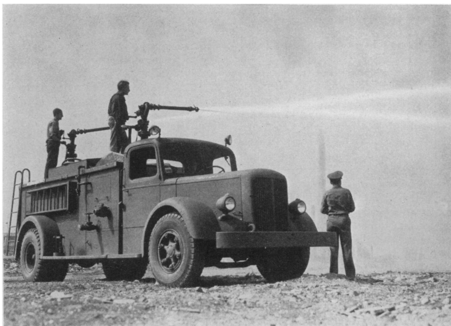
CRASH TRUCK —Built for Army Air Forces, this truck is ready to rush to the scene of a crash and shoot hundreds of gallons of water on a burning plane, blacking out the fire and rescuing pilot and crew. Engineers of Mack Trucks, Inc., worked with the Fire Prevention Section of the U. S. Corps of Engineers in developing the unit.
