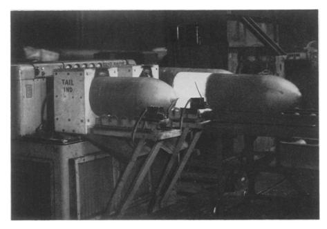
CONCENTRATED HEAT—In just three minutes and 15 seconds, the tails of these 500-pound bomb casings were heated to a 2,000-degree white heat at Wheeling Steel. The heating is done so quickly in an induction furnace that the front end remains cool enough to handle without tongs. The concentrated heating is made possible by the use of electric induction furnaces made by Ohio Crankshaft Company.
