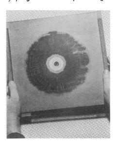
coated with lacquer. The circular pattern of tiny cracks which results is dyed to make the pattern more prominent, as shown in the picture. These tell-tale "footprints" are studied by engineers to aid development of better armor plate and better armor-piercing shells. The method is expected to have peacetime use for locating strains in machin-
