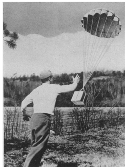
LOADED — Parachutes of wet-strength paper to deliver food and supplies to our armed forces were developed by the U. S. Navy Department with the cooperation of Dennison Mfg. Co.
