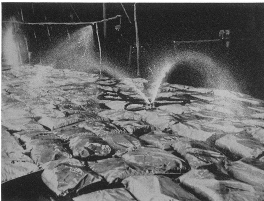
DRENCHED —To test the ability of paper bags to withstand rough treatment, paper shipping sacks developed by Bemis Bro. Bag Co. and the American Cyanamid and Chemical Corp. were sprayed with water for 24 hours.
