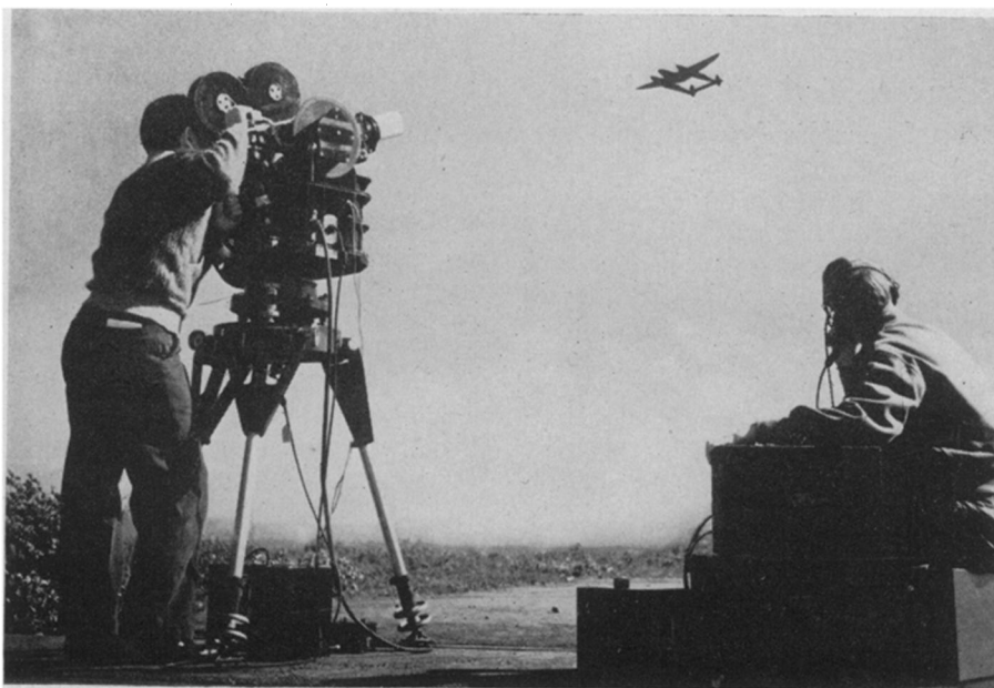
MOVIE CAMERA —This instrument, called a phototheodolite, was designed to facilitate the testing of airplanes during take-offs, landings, dives and other maneuvers involving a knowledge of flight path, altitude and velocity. The camera photographs the airplane, a time counter, and elevation and azimuth angle scales simultaneously. The operator's assistant, at the right, maintains contact with the airplane by radio. This is an official photograph of the National Advisory Committee for Aeronautics.
