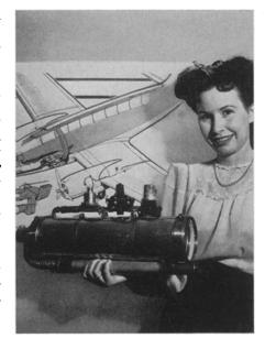
use is to de-ice windshields, prevent ice from forming on wings, and to keep bombsights, instruments and other equipment operating.
