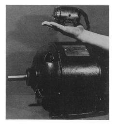
POCKET-SIZED—This midget motor, but one-fifteenth the size and weight of the average three-horsepower motor, operates at 120-000 revolutions per minute, or 65 times the speed of the motor of a household washing machine. It has been developed by the General Electric Co. for use in grinding and drilling airplane parts and other war equipment.
