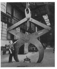
GIANT—This massive tong has a lifting capacity of 80 tons, weighs 12,489 pounds itself and has an opening 69 inches wide. Constructed by Heppenstall Co., Pittsburgh, it was specifically designed for use in handling ingots in a steel plant. The small tong between the claws of the larger one has a lifting capacity of 1,600 pounds.
