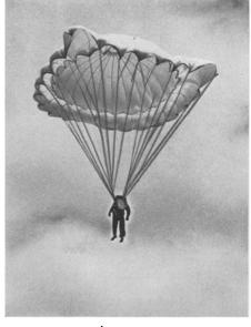
controlled slots which extend from the parachute canopy are manipulated by the jumper, who can thus select a landing place. Photograph shows the chute in
