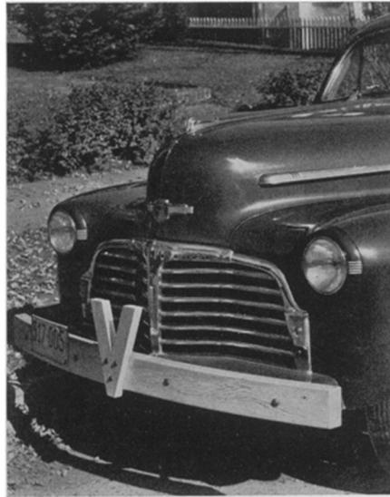
picture, made of five-ply laminated wood, is as serviceable as ordinary metal bumpers.
