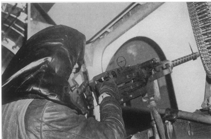
MODERN KNIGHT —This latest flak helmet designed to protect the head and neck of aerial gunners is made up of many small metal squares and is lined with sponge rubber to reduce shock and concussion. Head and neck wounds, suffered by 25% of air casualties, should be greatly reduced by this headgear. Official U. S. Army Air Forces photograph.
