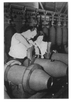
HEAVY PAPER rings or "wheels" encircling heavy aerial bombs ready for shipment are shown in the picture. A synthetic ureaformaldehyde resin makes the paper tough and waterproof enough to withstand rain and snow, and also shock-resistant. Replacing steel, the paper saves millions of pounds of the metal.
