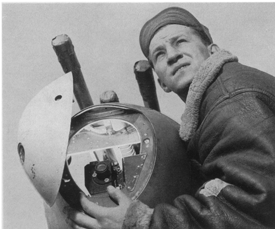
GUN-CAMERA TEAM —The nose of a P-38 airplane has been opened to show you the camera installed there by Materiel Command experts of the Army Air Forces to photograph enemy planes at the instant that they are being shot down by the guns above. This is an official photograph.
