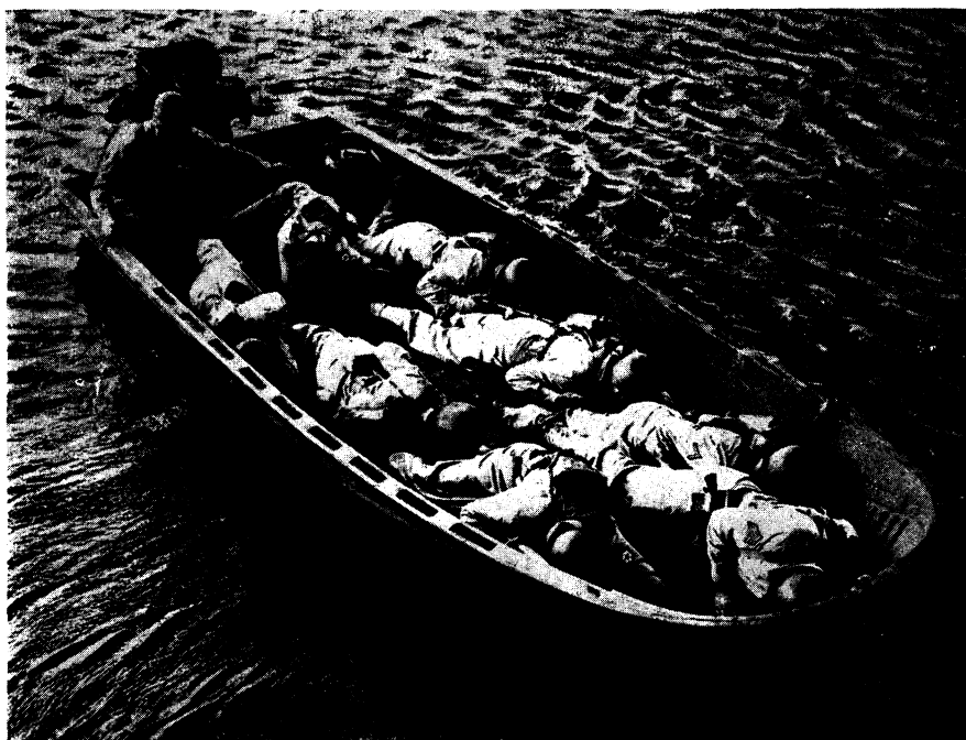
STORM BOAT —Making themselves as small as possible to reduce the target and lower the center of gravity, a squad starts for its objective in the new plywood craft of the Army.
