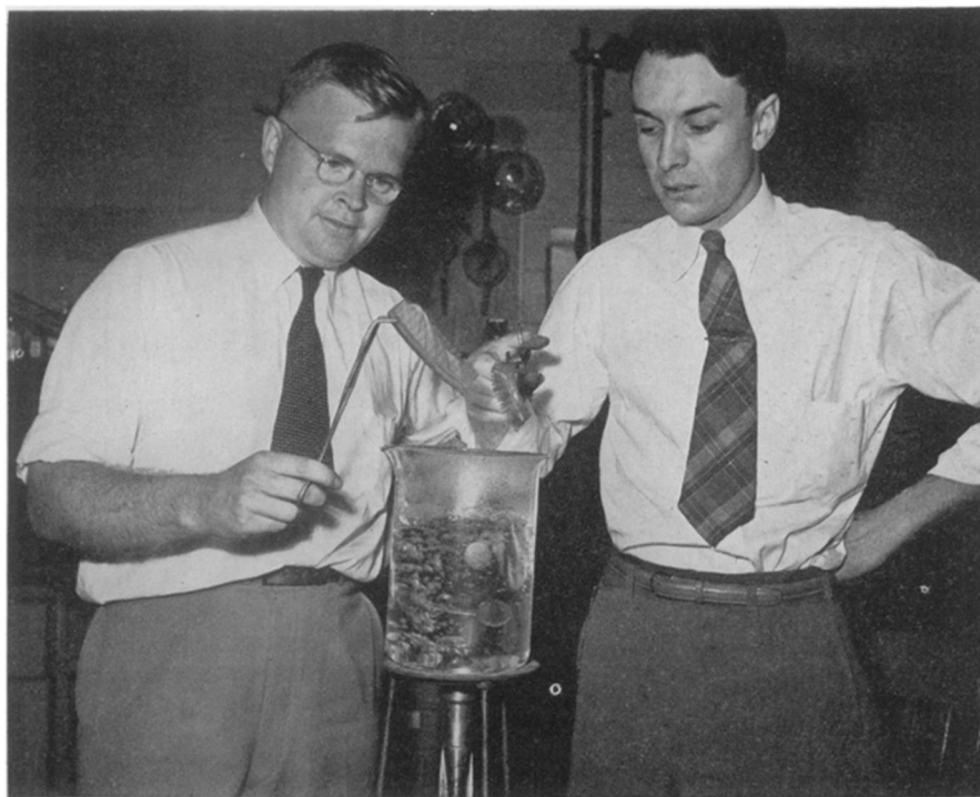
HEAT RESISTANT —Dr. Reid Fordyce and Dr. David Mowry illustrate the advantages of the new plastic, Cerex. Here you see two combs which have been dipped into boiling water. The one on the right is of ordinary plastic, the other of Cerex.
