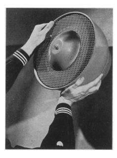
about 25 pounds. The illustration explains its nickname, the "salad bowl." Its base contains a transformer. The magnetic unit is fitted with a two-piece permanent magnet.
