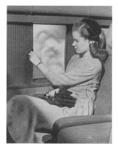
AIRPLANE window closure for passenger planes after the war operates horizontally as shown in the illustration. With it a passenger can screen all or part of the window.
