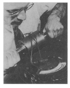
to determine, and so regulate, the power output of his engines accurately. It measures the minute twist in the shafts between engines and propellers, and through this the amount of driving force delivered. The picture shows a model, sensitive enough to measure the twist of a steel rod distorted by the hands.
