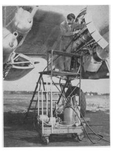
PORTABLE PRE-OILER—This compact device delivers pre-heated oil under pressure to the engines of B-26 Marauders. Developed at the Glenn L. Martin Company, it has demontrated its value both as a saver of man hours and a preventer of failures due to improper lubrication of an engine prior to its first start.
