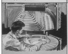
ELECTRONIC CHEMIST...The Westinghouse Mass Spectrometer analyzes intricate gas mixtures at amazing speed. In making synthetic rubber, for example, this electronic device cuts the time of chemical analysis from days to a matter of minutes.
