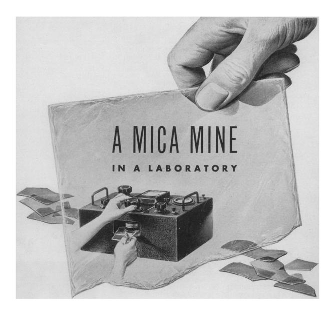
War shortages crop up in strange materials. Mica, for instance. Once seen principally in the windows of stoves, and in boys' pockets, it is now used extensively as electrical insulation. In some products, it is almost indispensable: capacitors for radio, spark-plugs for airplane engines, insulators in electronic tubes.
