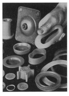
SYNTHETIC RESIN called compar is replacing rubber in certain washers, seals, gaskets, diaphragms and other flexible articles because of its elasticity, flexibility and abrasion resistance. The articles, as illustrated, are molded of this vinyl resin derivative into various shapes.
