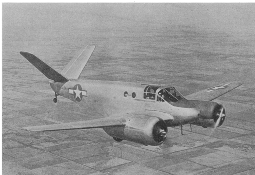
BUTTERFLY TAIL —Stability and control characteristics of this V-tailed Beechcraft are rated "excellent" by test pilots who have flown it.
