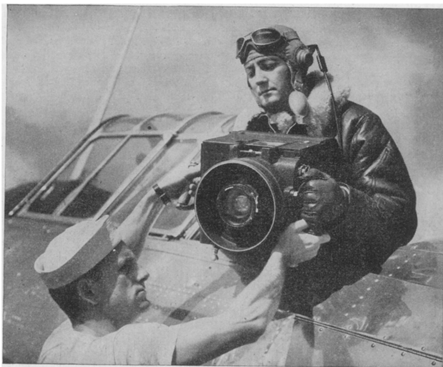
B&L Altimar f:4 lens in Fairchild (F-56) Aerial Camera.
