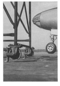
SAFETY LADDER for mechanics working on planes on airfields can not "creep" when fitted with metal brackets behind the wheels on its front support, as shown in the picture. When the ladder is tipped forward to be moved to a new position the wheels come in contact with the ground.
