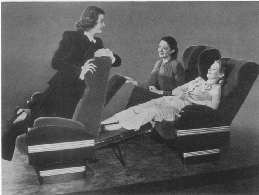
POSTWAR COMFORT —A button in the chaise lounge seats designed by Pullman releases a leg rest from the seat ahead, providing full-length comfort.
