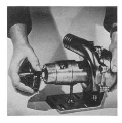
of water a minute and requires but one horsepower to operate. Based on the principle of the Archimedes screw similar to the worm in the familiar meat grinder, it has two screws with a step between.
