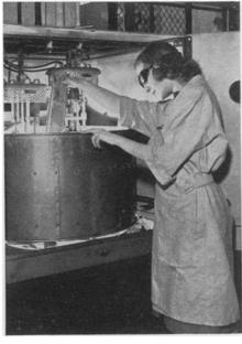
thetic rubber-like fabric. With the instrument, illustrated above, the effects of sunlight, periodic rain and temperature changes on the material can be determined in advance.
