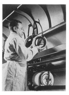
TOUGH TIRES—Chemicals used in compounding rubber are ground and mixed in this ball mill at the Firestone Tire and Rubber Company's research laboratory. The chemicals (also called compounds or pigments) are ground up by the stones as the jars turn on rubber rollers in the mill.
