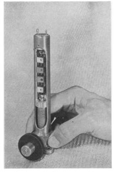
VIBRATRON, shown in the picture, is a new precision instrument versatile enough to help in many industrial problems, including measuring a wide range of physical qualities such as temperature and pressure, and in the audio-frequency field. A stretched wire in an electro-magnetic field is the actuating element.
