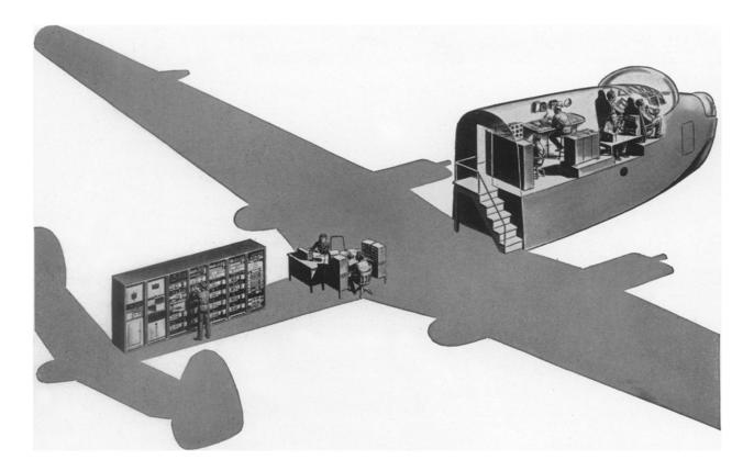
This is a "flight trainer"—an electronically operated replica of the PBM-3 flying boat. It was conceived by the Bureau of Aeronautics and developed by Bell Laboratories to train Navy crews on the ground.
