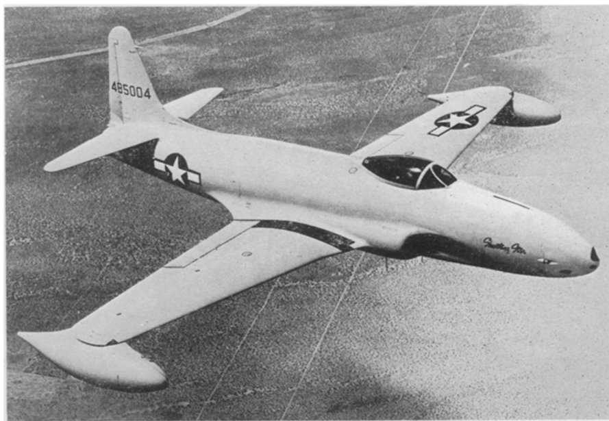
JET FIGHTER —Shown in flight is the U. S. Army Air Forces' new P-80 Shooting Star. The plane is powered by a new jet propulsion gas turbine engine and is capable of speeds in excess of 550 miles per hour. The service ceiling is above 40,000 feet.
