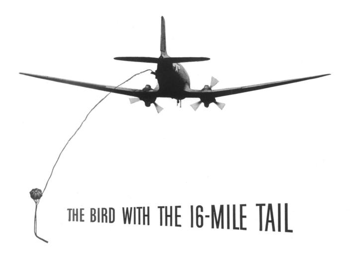
The wire you see with the parachute on the end of it is a telephone wire, being payed out from a C-47 plane.
