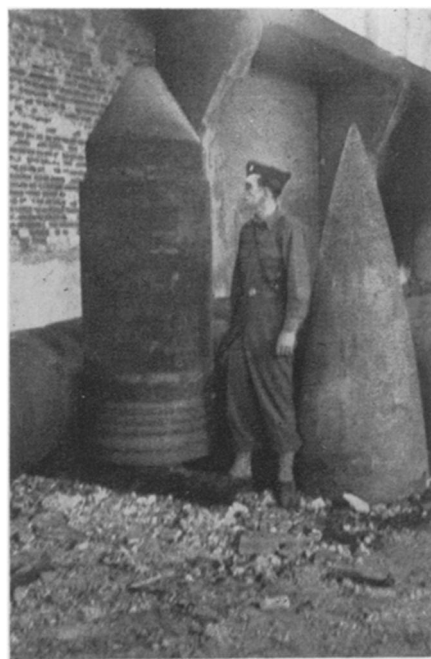
COMPARISON —The man appears dwarfed beside the huge projectile. The weight of the projectile plus windshield is eight tons; over-all length is 13 feet.
