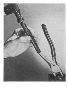
mered onto the handles without cracking or splitting. Being of non-conducting material they provide insulation for work on electric lines.
