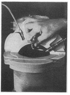
B-29'S SUCCESS—In the new Bendix-Stromberg direct fuel injection system, which equipped the Superforts that dropped the atom bombs, the fuel is pumped under pressure directly into individual engine cylinders, entering via the stainless steel fuel lines and the nozzle shown at the upper left. Spark plug is at right. The technician's hand holds the fuel spray nozzle at the point where gasoline is sprayed into the cylinder.
