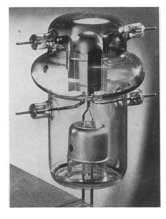
communication equipment, have two identical small filaments mounted in lock-in type bases, one of which is shown in the picture. One filament carries the high-frequency current, the other an ordinary current regulated until both filaments are equally bright.
