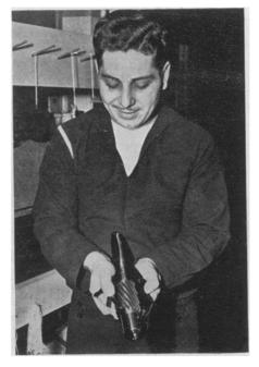
transmits a minimum amount of moisture. To remove, the plastic is slit with a knife and stripped off as illustrated in the picture.
