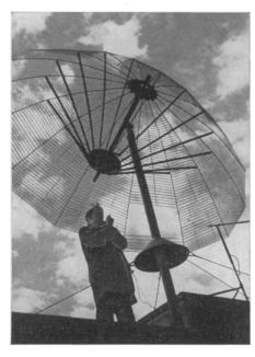
🌣 RADAR UMBRELLA, a light portable unit developed especially for beachhead use, is used both as a reflector in sending out shortwave radio pulses and as a receiver to catch wave echoes reflected from enemy targets. The unit's rotating umbrella-like antenna is shown in the picture.
