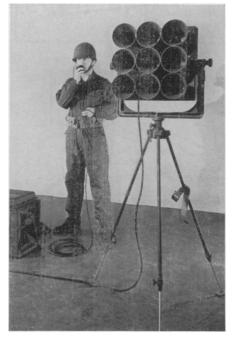
d LOUDSPEAKER, powerful enough to pierce the thunder of battle, has nine receivers and horns mounted on a common panel pivoted on a tripod so that it can be turned up or down, to right or left. Horns, tripod and operator are shown in the picture.
