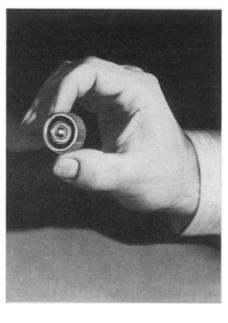
Signal Corps has now been developed into the commercial model shown in the picture, used principally in hearing aids. Chemical reaction of zinc and mercuric oxide operates the cell; conventional cells use zinc and carbon.
