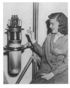
ELECTRONIC TUBES, the most powerful ever built and the smallest ever made, are shown in the picture side by side for comparison. The 200-kilowatt giant weighs 80 pounds and is used in government transmitters for beamed overseas broadcasts. The midget is a hearing-aid tube, 0.7 ounce in weight.
