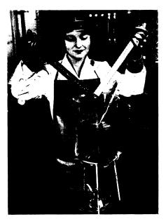
RESISTS ACIDS—From a boiling bath of hot sulfuric acid, a laboratory technician lifts two rods of plastic. One has charred and deteriorated. The other, made of Du Pont's new "Teflon" tetrafluoroethylene resin, is not affected at all by the highly corrosive acid. "Teflon" is not attacked even by aqua regia, which dissolves gold and platinum.
