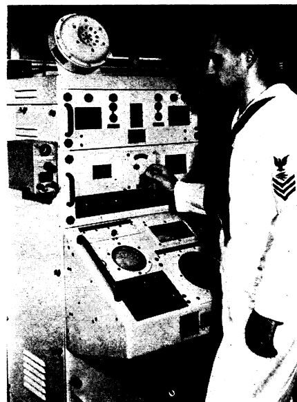
DEFEATED SUBS —This is a side view of the sonar control console, test installation, with operator tuning equipment. Controls are grouped in an assembly called the Stack, usually located in or near the pilot-house. Official U. S. Navy photograph.
