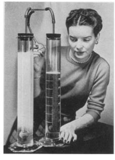
ANTI-FOAM agent prevents oil in high-speed engines from bubbling and frothing due to air-mixture. The picture shows the effect when air is forced through treated and untreated oils. The agent, composition still secret, reduces surface tension on each individual bubble as formed, causing it to break quickly on reaching the surface.
