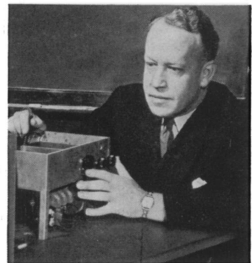
Stuart William Seeley, Manager of the Industry Service Laboratory, RCA Laboratories Division, perfected this new FM circuit. It not only operates equally effectively with strong or weak stations, but lowers the cost of receivers by eliminating additional tubes and parts that were formerly considered necessary in Frequency Modulation receivers.
